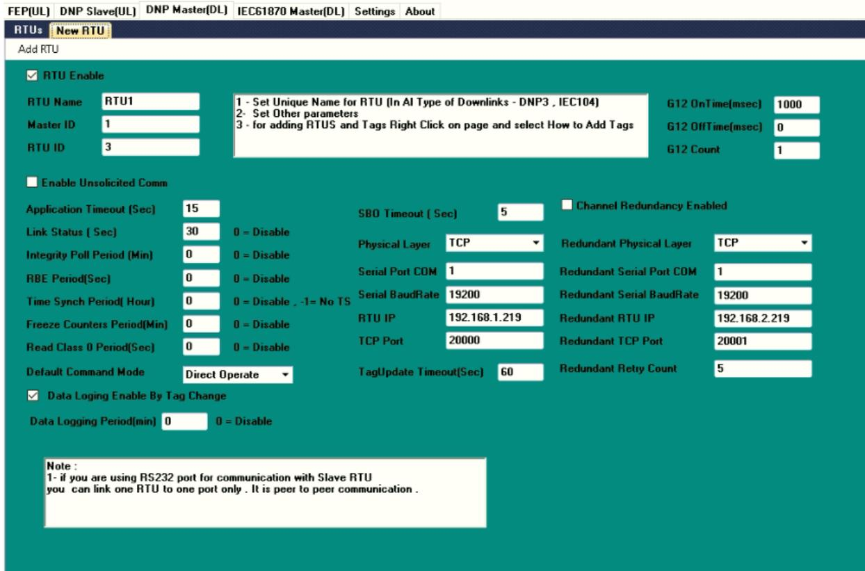
The screenshot shows the 'New RTU' configuration page. At the top, there are navigation tabs: FEP(UL), DNP Slave(UL), DNP Master(DL), IEC61870 Master(DL), Settings, and About. Below these is a sub-header 'RTUs: New RTU' and a title 'Add RTU'. The main configuration area is divided into several sections:
