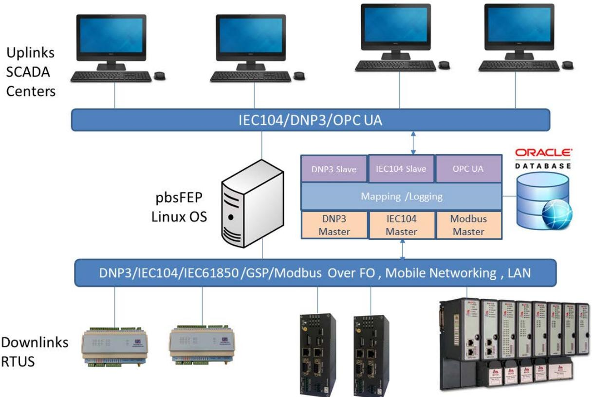
Downlink connections, are RTU Connections. Downlink Connections in pbsFEP are TCP Client Connections. DNP3 Master, IEC104 Master, Modbus Master are samples for Downlinks connections.
