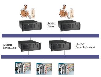
pbsHMI supports warm Server redundancy structure and in a bump less operation clients and PLC/RTUs are switching between Servers.
