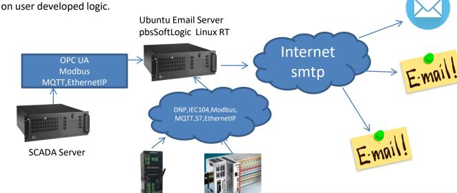
The mail server can be a standard Ubuntu server with the pbsSoftLogic runtime kernel installed. Email server can read data from SCADA server or directly from RTU with various supported protocols such as DNP3, IEC104, OPC UA, Modbus, MQTT, Redis, S7, AB, ....
