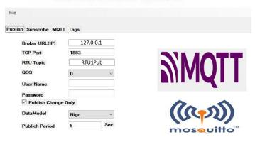
There is a GUI for each communication driver for easy configuration. DNP3, IEC101/104, Modbus, Fatek PLC, Vestas Wind Turbine, IEC62056-21 and IEC62351 and GSP are developed at pbsControl.
