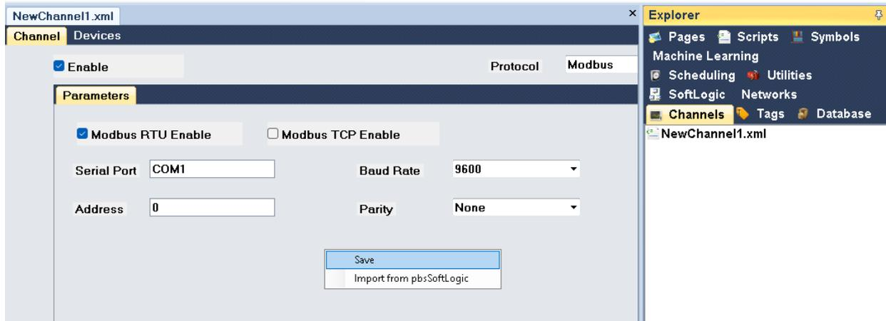
Right click in the channel setting page and save settings. Close “NewChannel1.xml” Setting page and right click on the channel list panel and run “Explorer” item. This will open channels folder in the project folder.
